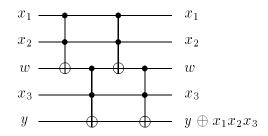
Again, we can eliminate the last gate if we don't mind flipping the value of the scratch bit.
