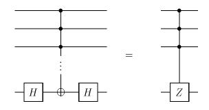
after conjugating the last bit by  $\boldsymbol{H}, \theta^{(n)}$  becomes controlled<sup>(n-1)</sup>- $\boldsymbol{\sigma}_z$ , which flips the phase of  $|11...|1\rangle$  and acts trivially on all other computational basis states. Conjugating by NOT<sup>(n)</sup>, we obtain  $\boldsymbol{U}_s$ , aside from an irrelevant overall minus sign.
