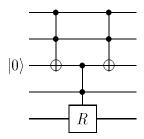
uses one scratch bit to construct a four-bit Deutsch gate ((controlled)<sup>3</sup>- $\mathbf{R}$ ) from the three-bit Deutsch gate and two three-bit Toffoli gates, and a similar circuit constructs the *n*-bit Deutsch gate from a three-bit Deutsch gate and two (n - 1)-bit Toffoli gates. Once we have an *n*-bit Deutsch gate, and universal classical computation, exactly the same argument as above shows that we can reach any transformation in  $SU(2^n)$ .
